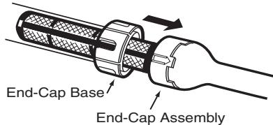
3. Grasp the black band at the base of the screen. **Do not grasp the filter screen.** Gently rotate the End-Cap Assembly toward you (about 1/8 turn) until you feel it stop.
