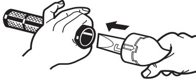
5. Line up the notches on the inside of the black band with the locking tabs on the End-Cap Assembly; slide the filter
